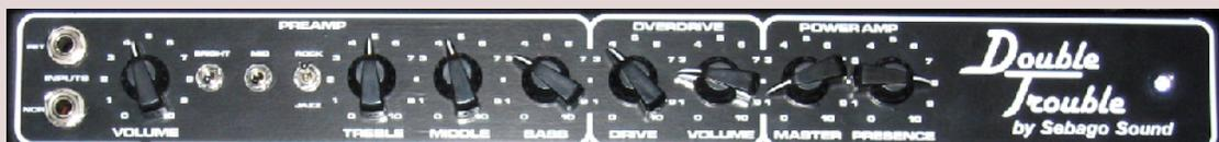
The first Volume control in the preamp section sets the level of the clean channel.
